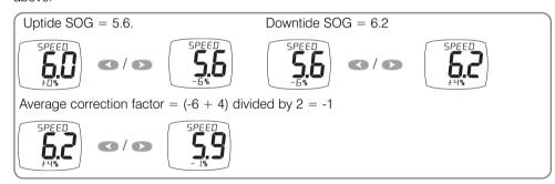
If you are unable to carry out this procedure due to strong tides or poor GPS data, go to www.raymarine.com for information on speed calibration using a measured distance.
